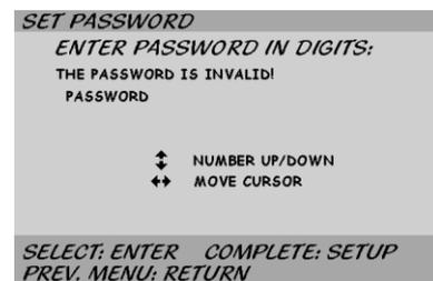
12. If the password is incorrect, the screen will return a password error message. In the Password Set screen are three fields, namely “REMOVE”, “CHANGE PASSWORD”, and “CHANGE RATING LEVEL”.
